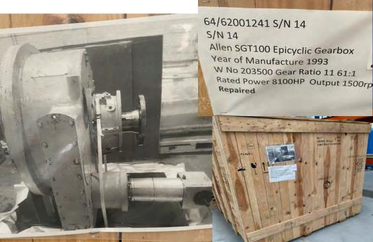
Lot 239 64/62001241 1x Allen Gears SGT100 Epicyclic Gearbox – Repaired W No 203500 Gear Ratio 11 61:1 Rated Power 8100HP Output 1500rpm Price £50,000
