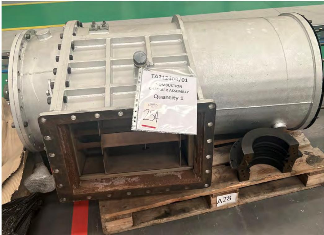
TA21240B/01 1x Combustion Chamber Assembly
