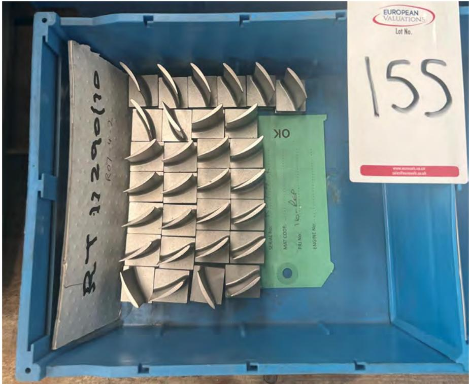
RT11290/10 30x Compressor Rotor Blade Stage 10
