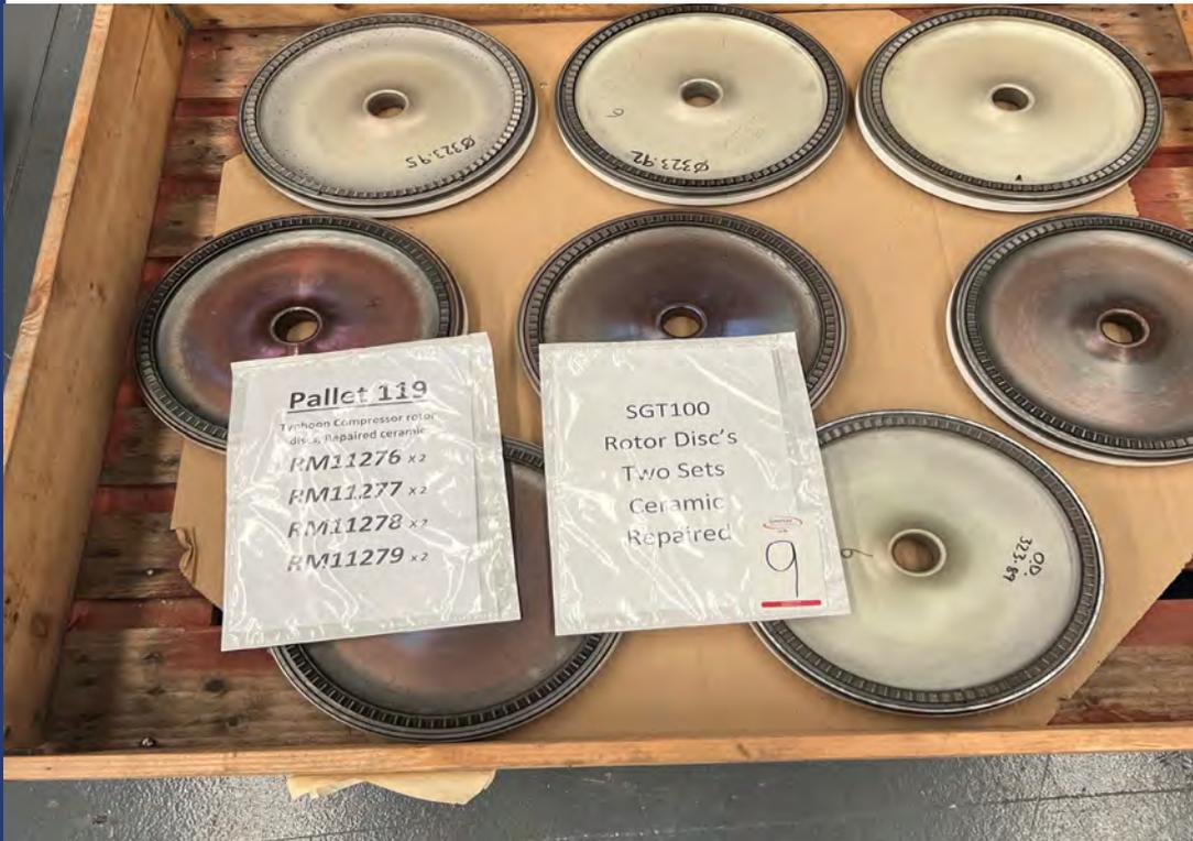
RM11276 2x Typhoon Compressor Rotor Disc - Repaired
